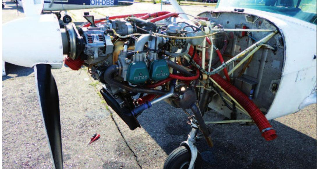
An important element of the kit is the engine adapter.
