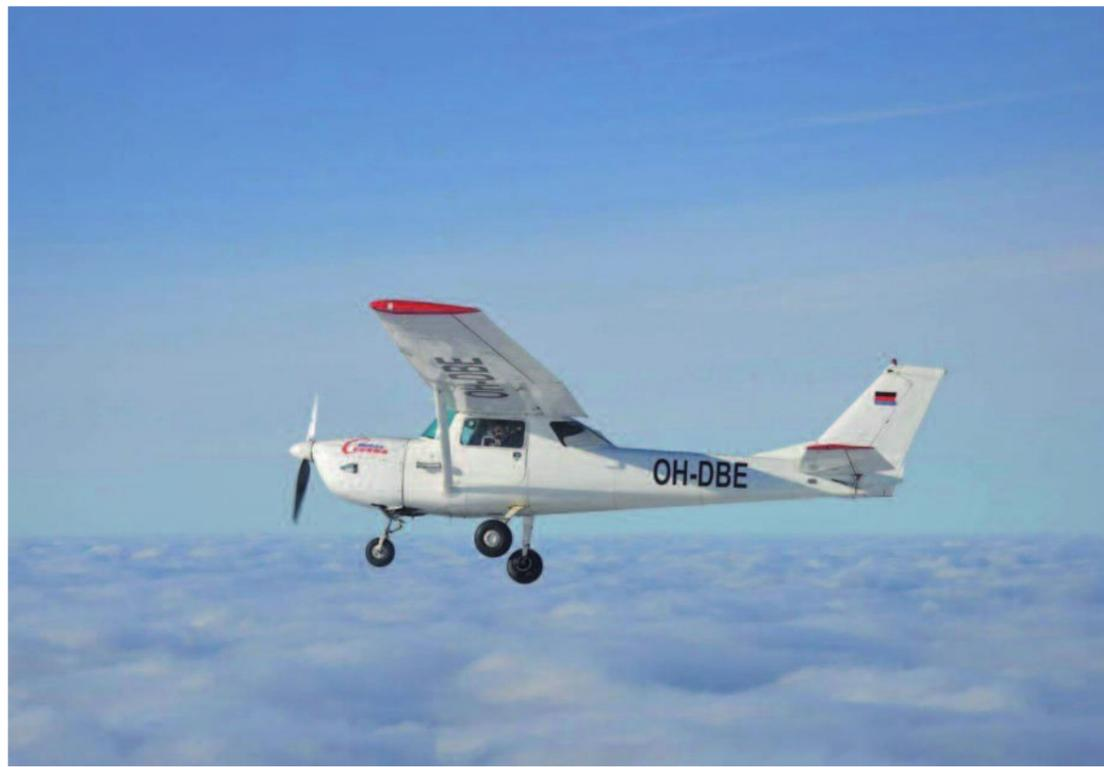
At first glance, the modified Cessna differs from the standard one by the greater length of engine cowlings
